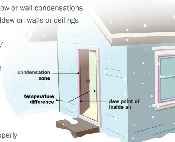
When warm, moist air inside the house touches a cold surface, the water vapor in the air turns to liquid water (condensation).
